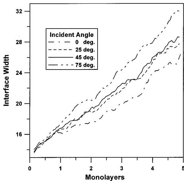
FIG. 9. Interface width variation at incident angles of 0°, 25°, 45°, and 75°, and the other conditions remain the same: 2 eV incident energy, 300 K substrate temperature, and 0.1 atom/ps deposition rate.
